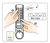
a Press 1, # and 5 buttons simultaneously for 4 seconds
