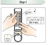
Press 1, # and 5 buttons simultaneously for 4 seconds
