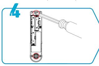
Open the door and loosen the screws and nuts on the back of the door to remove the product.
