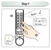
Press 6, # buttons simultaneously for 2 seconds
