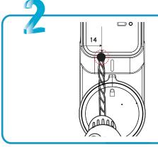
Drill the hole horizontally to the point where it should be drilled.
