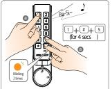
Press 1, # and 5 buttons simultaneously for 4 seconds
